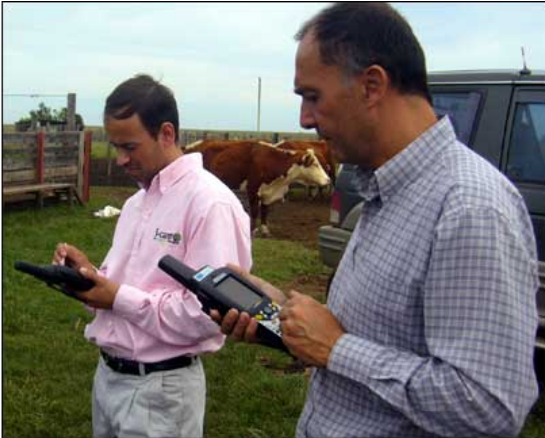
Participants in Uruguay's cattle-tracking pilot are using Psion Teklogix PDAs with Agrident RFID readers to identify cattle as they move from one location to another.
